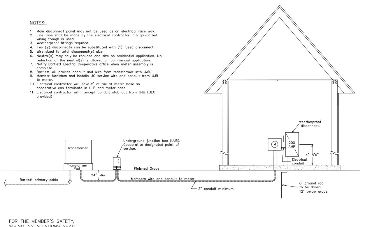
FOR THE MEMBER'S SAFETY, WIRING INSTALLATIONS SHALL CONFORM TO THE REQUIREMENTS OF THE NEC AND NESC.
