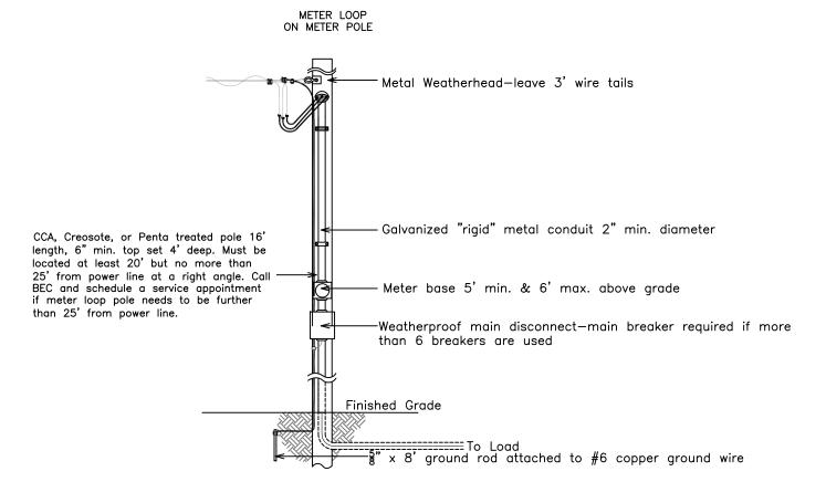
FOR THE MEMBER'S SAFETY, WIRING INSTALLATIONS SHALL CONFORM TO THE REQUIREMENTS OF THE NEC AND NESC.
